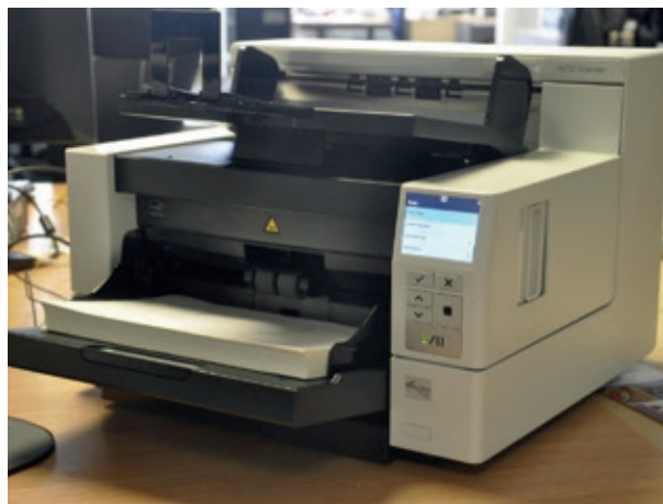
Fig. 4 Document scanner for destructive scanning
