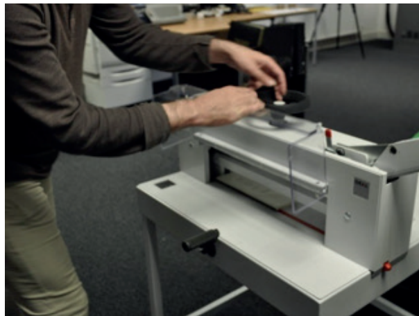
Fig. 3 Spine removed for destructive scanning
